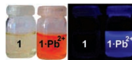
Figure 6. Visual features observed in \text{CH}_3\text{CN} solutions of 1 and \mathbf{1}\cdot\text{Pb}^{2+} . Left, absorptions; right, emissions.
